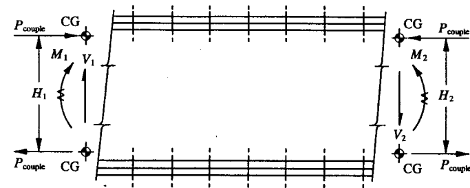
FIGURE 4-4 Isolated segment of beam in equilibrium. Internal loads shown at exposed sections of beam.
